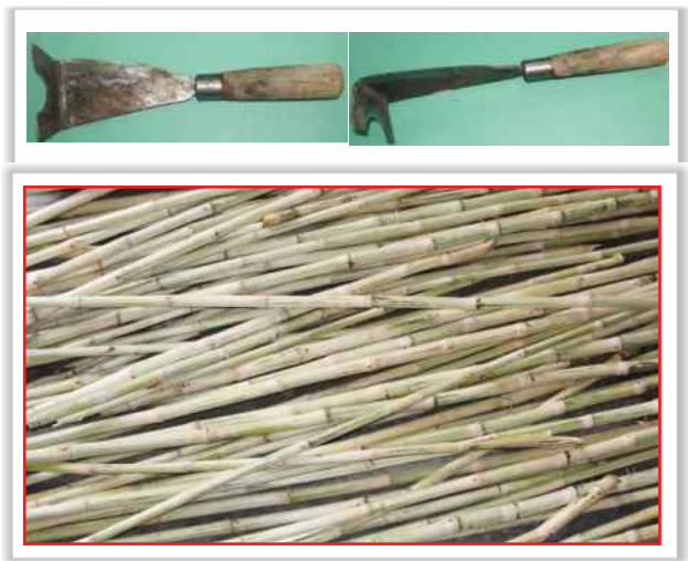
Fig. 7.2. Sugarcane scrapper-cum-cutter and cleaned canes after its use
