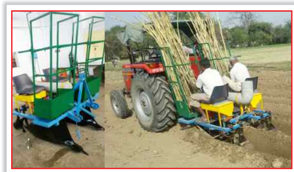
Fig. 6.1. Tractor operated deep furrow sugarcane planter
