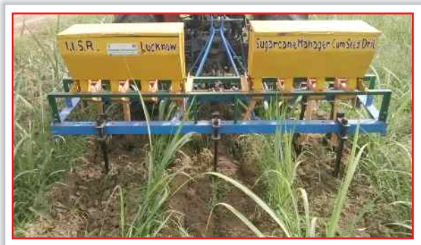
Fig. 6.3. Tractor operated sugarcane manager with fertilizer application and sowing arrangements
