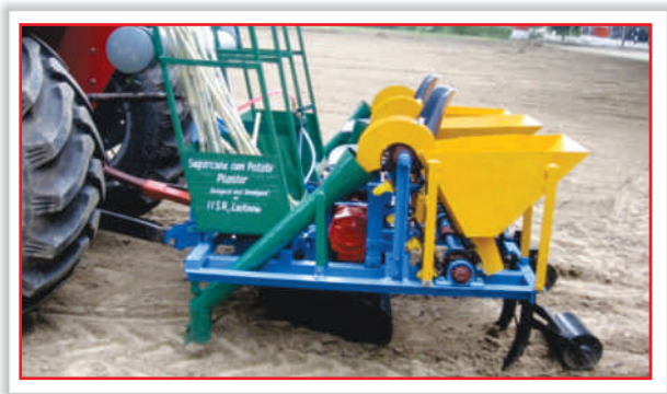
Fig. 6.4. Modified tractor operated sugarcane-cum-potato planter
