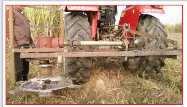
Fig. 6.5. Tractor operated rear mounted sugarcane harvester
