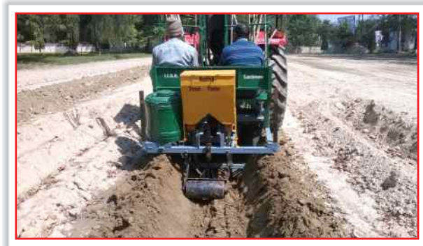
Fig. 6.2. Modified sugarcane trench planter
