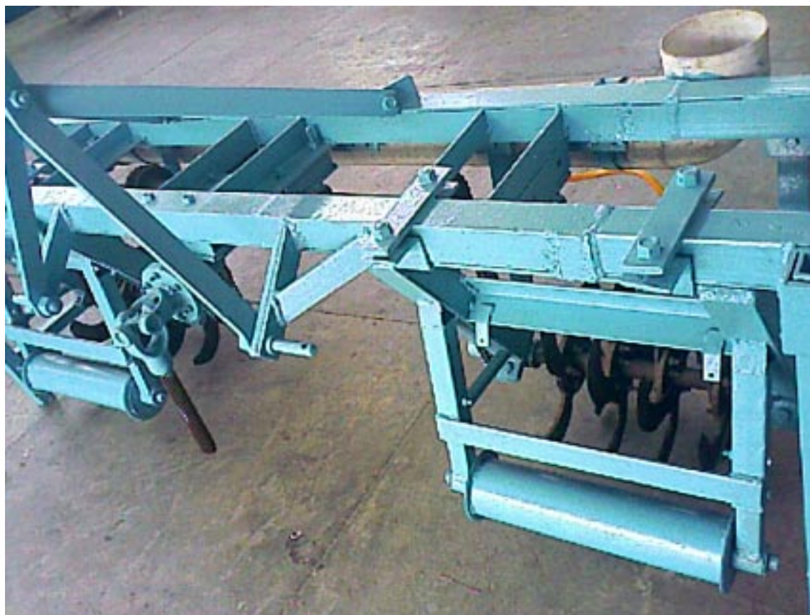
Plate 7.5. Residue mulcher-cum-bio applicator
