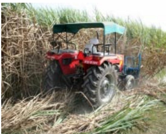
Plate 7.1. Tractor operated front mounted sugarcane harvester in operation
