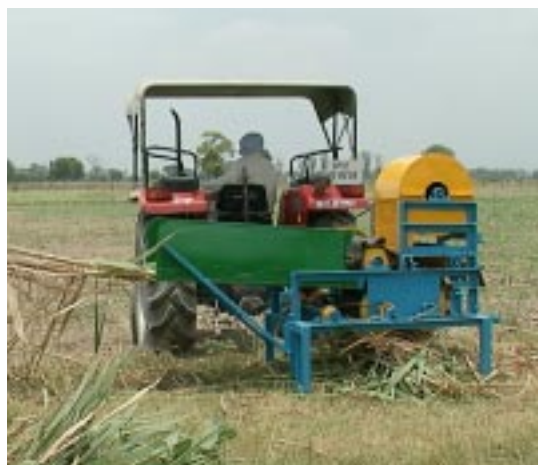
Plate 7.3. Sugarcane detrasher in operation
