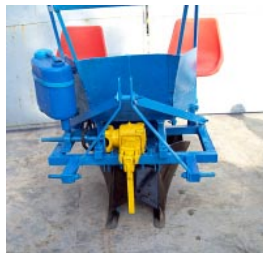
Plate 7.4. Front view of wide spaced paired row sugarcane cutter planter
